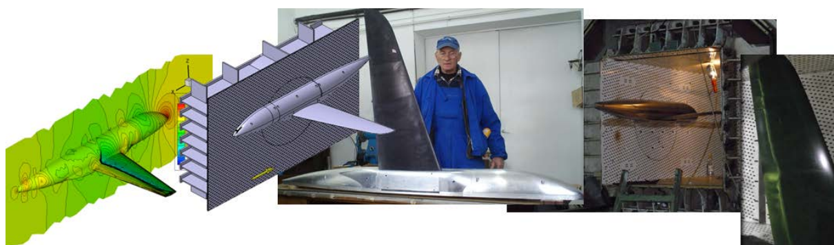
Fig. 4 – Buffeting alleviation technology demonstrator in INCAS Supersonic Wind Tunnel
